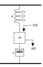
The goal is to view the position x(t) of the mass m with respect to time t. You can calculate the position by integrating the velocity of the mass. You can calculate the velocity by integrating the acceleration of the mass. If you know the force and mass, you can calculate this acceleration by using Newton's Second Law of Motion, given by the following equation:
